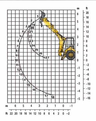
Lift Capacities are over-end values. Machine equipped with AWD, OROPS, 0.96 m<sup>3</sup> (1.25 yd<sup>3</sup>) general purpose bucket, and 250 kg (550 lb) counterweight. Extendible stick includes 485 kg (1,070 lb) counterweight.
